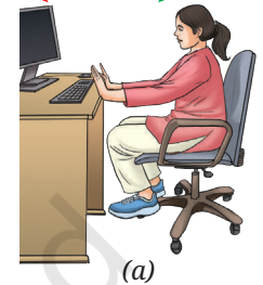
(a) Force applied by the girl on the table (red arrow) and Force applied by the table on the girl (green arrow)
