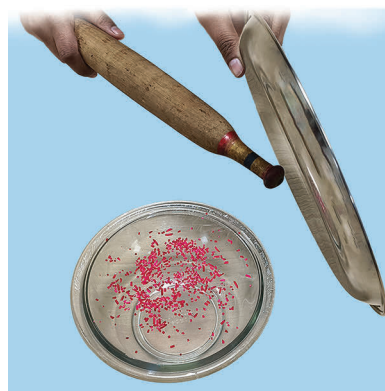
Fig. 10.14: Sound moving grains (coloured)
